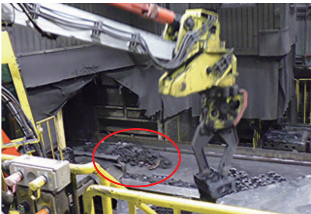
At the Kubota Okajima Business Center, we are working to reduce waste by improving the utilization rate of collection facilities for recycling waste casting sand generated in the product manufacturing process (in the red frame). This initiative reduced waste emissions by some 1,550 tons in FY2020.
