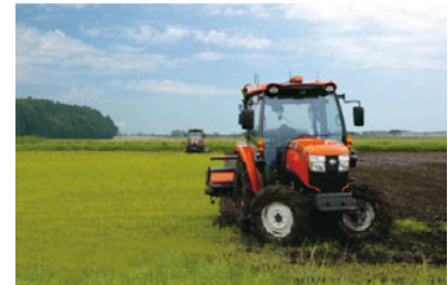
Test operation of one manned and one unmanned AGRIROBO tractor working in collaboration
