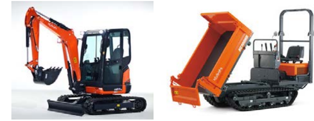
ZERO TAIL EXCAVATOR
