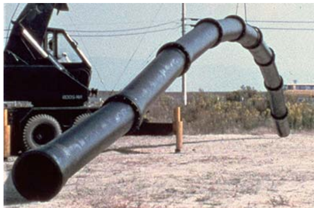
Hoisting test for a ductile iron pipe using earthquake-resistant joints
