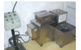
Promoting recycling through use of a waste thinner recycling unit
