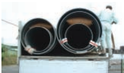
Improvement of load efficiency by collectively transporting smaller diameter pipe
