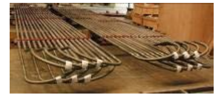
Cracking tubes for ethylene
