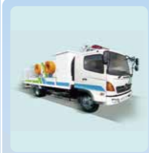
Drainage Pump with Vehicle
