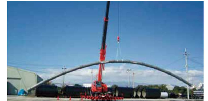
Hanging test of earthquake resistant joint
