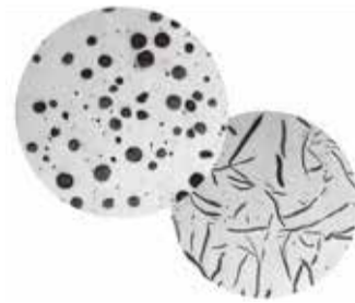
Microstructure of ductile cast iron (left) and cast iron (right).
