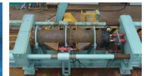
The pipes are tested by hydraulic pressure.
