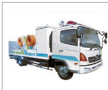
Highly maneuverable drainage pump vehicle
