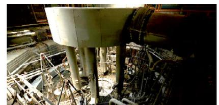
Rotary-type surface melting furnace that can liquefy residue and ash, turn it into slag, and reuse it as a resource
