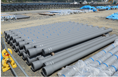
Ductile iron pipe (used in the restoration and maintenance of lifelines, such as water supplies, sewage lines, and gas lines)
