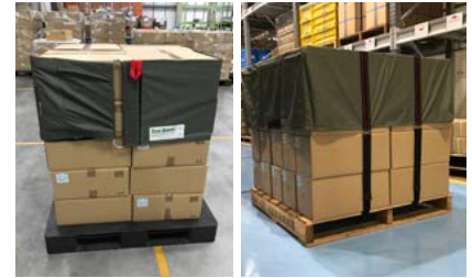
Returnable packaging materials (left: environmentally friendly strapping; right: environmentally friendly cover) KBS Kubota Co., Ltd.
