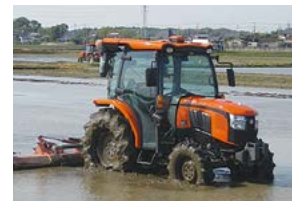
Agri Robo Tractor capable of performing unmanned automatic operations
