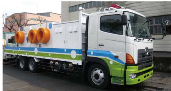
Drainage Pump with Vehicle for Disaster Recovery
