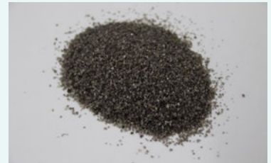
Soil conditioner made from water granulated slag as a raw material
