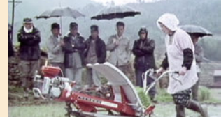
Fully automatic walk-behind rice transplanter, the original model for subsequent transplanters
