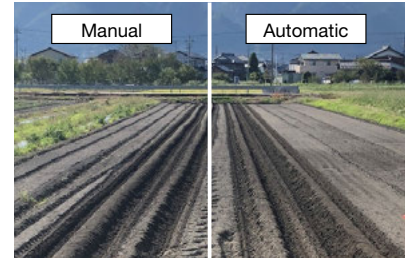
Straight-line test runs by GS-enabled Kubota GRANOVA Tractor (NB21GS) Left picture shows results achieved with manual steering, right picture shows results with automatic steering, both by inexperienced operators. System also substantially reduces workload for experienced operators by maintaining straight-line accuracy
