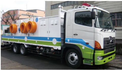
Drainage Pump with Vehicle for Disaster Recovery
