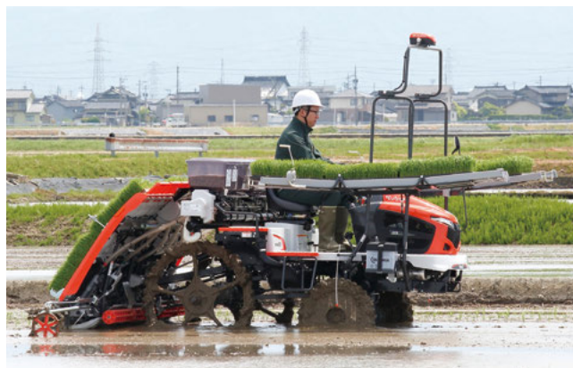
Rice transplanters: used to transplant rice seedlings to rice paddies, contributing significantly to labor saving.
