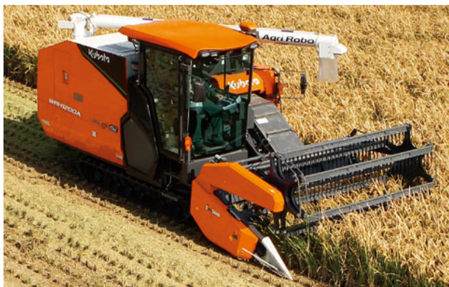
Combine harvesters: used for simultaneous harvesting and threshing of crops such as rice, wheat and pulses.
