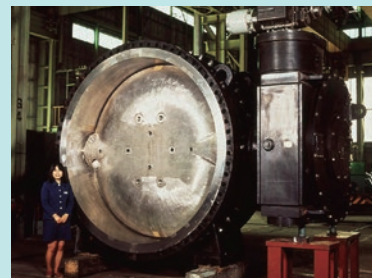
Stainless metal sheet 2400 mm butterfly valve delivered to the New York Water Bureau
