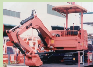
Full-revolving small hydraulic shovel (KH1), the base model for subsequent Kubota mini excavators
