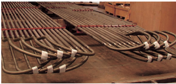
Steel casting: used at petrochemical plants for ethylene purification and other operations.
