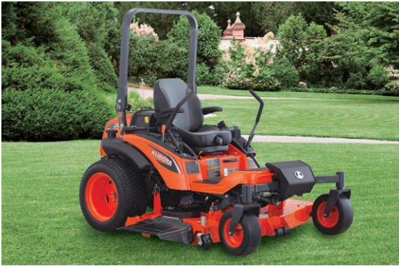
Riding mowers: used for cutting lawns in private residences, office areas and parks.
