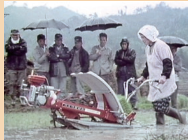
Full-automatic walk-behind rice transplanter (SPS type), the original model for subsequent transplanters
