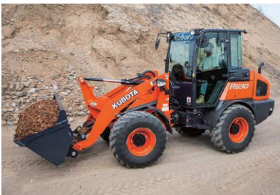
Wheel loaders: used mainly for transporting and stacking tasks (at construction sites, farms, etc.).
