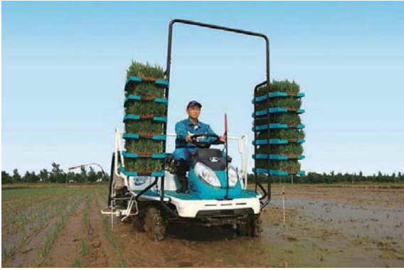
Rice transplanters: used to transplant rice seedlings to rice paddies, contributing significantly to labor saving.
