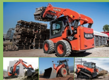
Above: Skid steer loader Below: from the left, mini excavator, wheel loader, compact track loader
