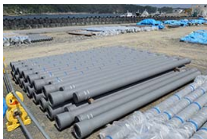
Ductile iron pipe This is used in the restoration and maintenance of lifelines, such as water supplies, sewage lines, and gas lines.
