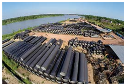
A stockyard for ductile iron pipes (φ900 - 1,200 mm)
