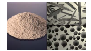
24 TXAX (brake pad material): used as a friction material, mainly in brake pads.
