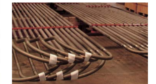
20 Cast steel: used at plants in the petrochemical industry for ethylene purification and other operations.
