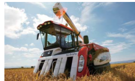
3 Combine harvesters: simultaneous harvesting and threshing of crops such as rice, wheat and pulses
