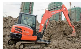
7 Construction machinery (mini backhoes): used in civil engineering and other operations; especially useful in narrow work areas, such as city streets.
