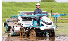
2 Rice transplanters: used to transplant rice seedlings to the rice paddies. Rice transplanters make a significant labor-saving contribution.
