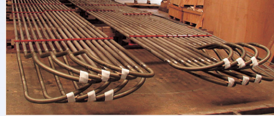
Cracking coils used in an ethylene plant
