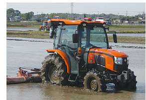
Agri Robo Tractor capable of performing unmanned automatic operations
