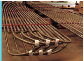
Steel castings Used at plants in the petrochemical industry for ethylene purification and other operations.
