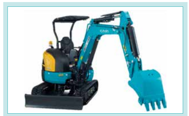
Fig. 2 A 3-Ton Class Tight Tail Swing Excavator U-30-6a
