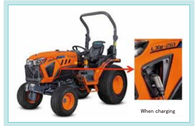
Fig. 13 Storage of Rapid Charging Inlet in Bonnet
