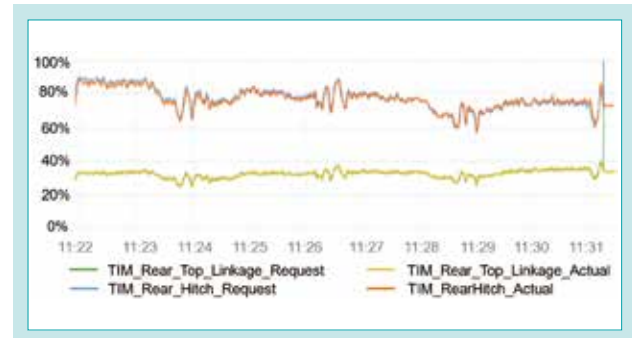
Fig. 8 Rear Hitch and Top Link Performances During the Field Tests Over the Time
