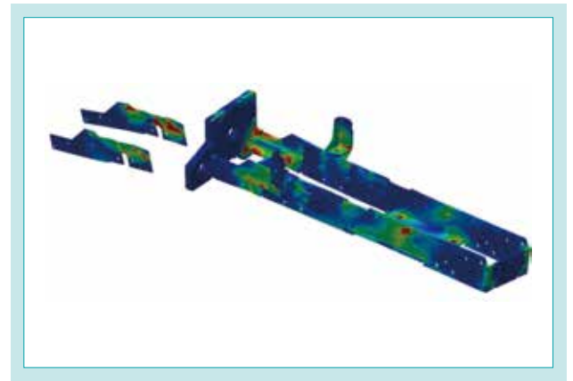
Fig. 7 Analysis Result of Frame after Improvement
