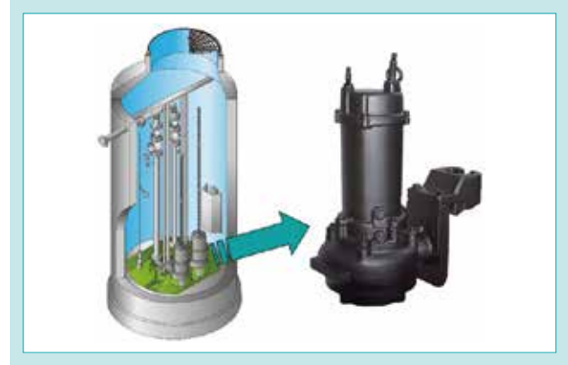
Fig. 1 Manhole Pump Unit and Submersible Pump
