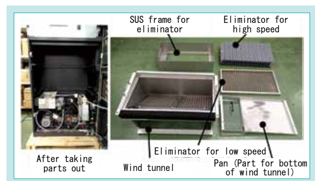
Fig. 10 Plumbing Component Parts
