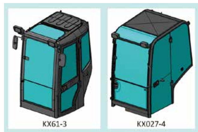
Fig. 3 External View of Cabin
