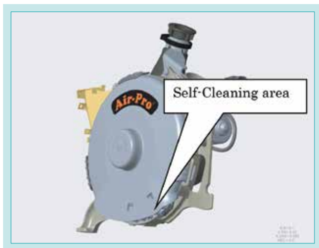
Fig. 10 Seed Meter with Improved Cleanout
