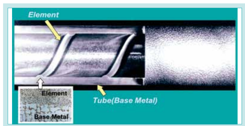
Fig. 3 Overview of MERT Cut Sample and the Microstructure
