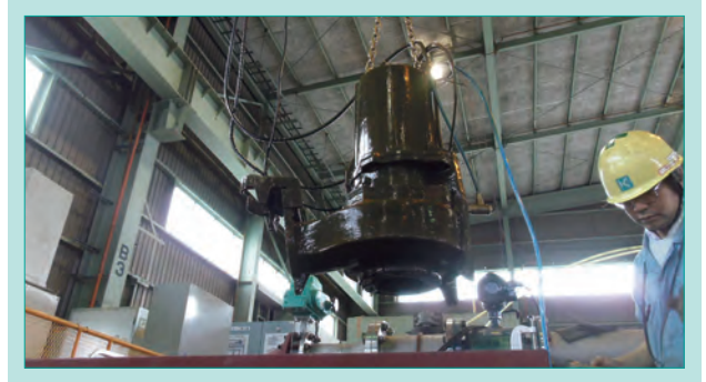
Fig. 9 Taking Out the Pump After Endurance Test
