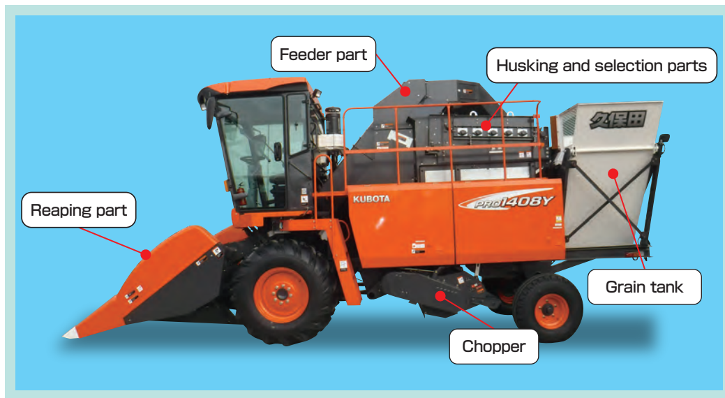
Fig. 3 Work Block of a Corn Harvester
