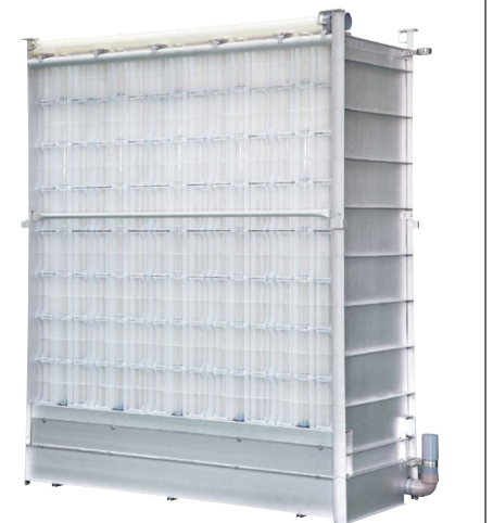
The KUBOTA Submerged Membrane Unit. Microorganisms degrade the wastewater into biologically treated water and solids (microorganisms) and then the membrane physically separates the treated water from the solids.
